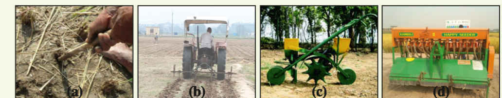
Fig. 3. (a) Hand seeding with stick, (b) Making marking by the tractor, (c) Star wheel planter and (d) Happy seeder.
